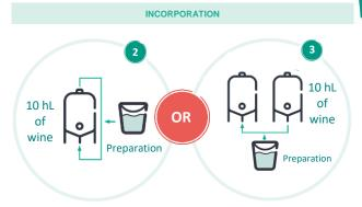
Homogenisation by reverse pumping over Add the solution with a Venturitype fitting. Homogenize well! Homogenisation by tank-to-tank transfer Homogenise well!
